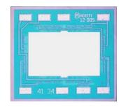
Stepped at: 1.8 mm in X and 1.6 mm in Y 77 columns by 84 Rows
